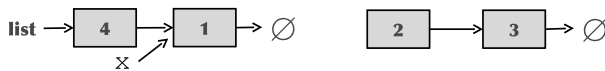
Figure 3.2: Linked list corruption. (a) code for push and pop, (b) starting data structure, (c) interleaving of pop and push, (d) final state. Items 2 and 3 are no longer on the list, and item 1 is both on the list and the return value from pop
